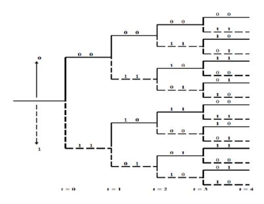
Fig.. Trellis diagram for the encoder in Fig. 3.1
