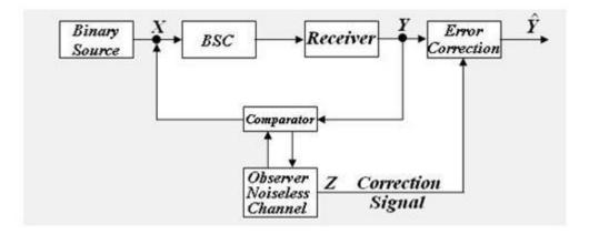
The observer is a noiseless channel that compares the transmitted and the received symbols. Whenever there is an error a \_ 1' is sent to the receiver as a correction signal and appropriate correction is effected. When there is no error the observer transmits a \_ 0' indicating no change. Thus the observer supplies additional information to the receiver, thus compensating for the noise in the channel. Let us compute this additional information .With P (X=0) = P (X=1) = 0.5, we have:
